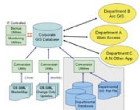
Figure 1. Logical overview of a corporate GIS datastore incorporating MasterMap and departmental Spatial data
