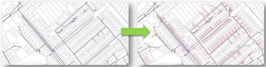
Using rules derived from UU business experts, 1Spatial inferred missing clean water assets with position based on buildings, live asset locations.
