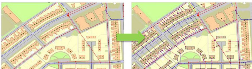
Additional more complex rules were derived by UU and 1Spatial for the inference and direction of missing Surface, Foul and Combined waste water assets.
